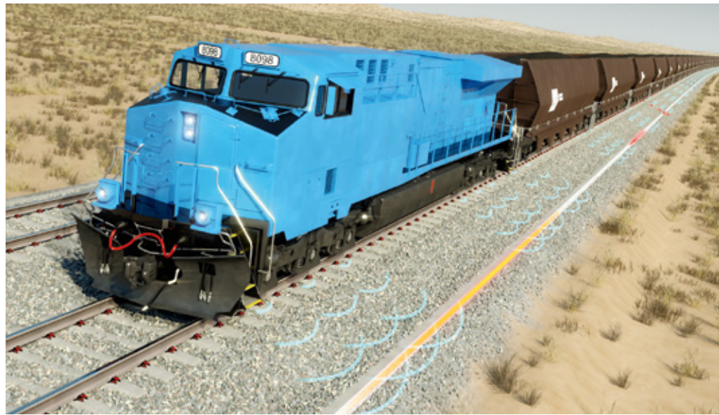
FIG. 2: By continuously monitoring the acoustic signature of the wheel-rail contact, the FTS support condition based maintenance strategies
