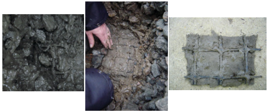
FIGURE 3: Geotextile or composite does not stop fine particle migration to the surface (reference: Ground Control)
