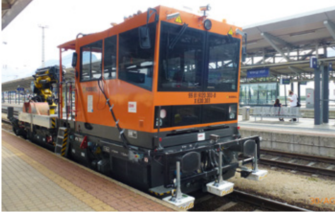
FIGURE 2: Figure 2: Antenna mounted on the train buffers of a maintenance vehicle (reference: Ground Control)
