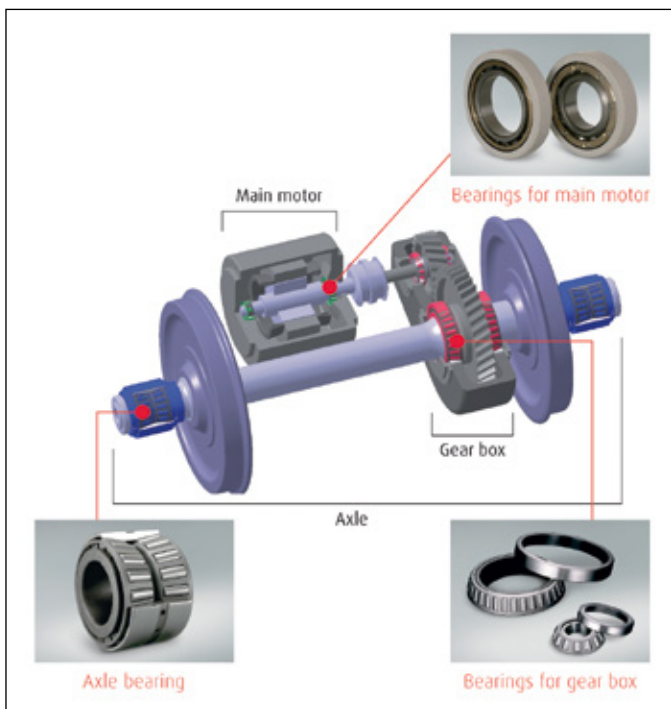
FIGURE 1: Axle of a current Shinkansen high speed train with main bearings
