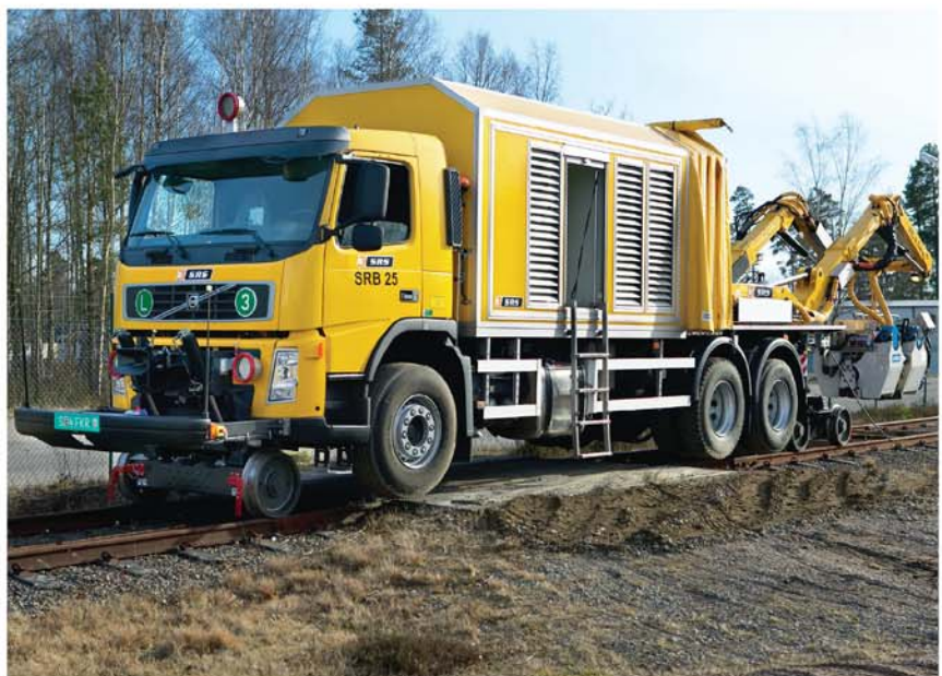
Road-rail vehicle for flash-butt welding
