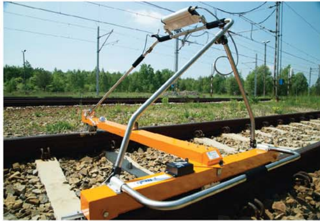
Track geometry measurement system TEC
